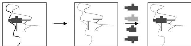
FIGURE 1 A MIP with the imprint molecule present (starting at the left side), removed leaving behind the receptor site and selected from a mixture of possible molecules.
